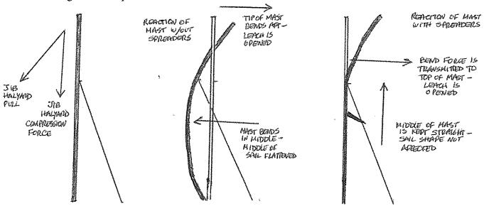
Masts equipped with spreaders allow more control over where precisely the bending of the mast takes place along its length. The swept back orientation of the spreaders and their location in the upper third of the mast combine to move the point of maximum mast bend upwards. This means that mast bend due to rig tension tends to affect the upper part of the sail, rather than the lower area. Again, this becomes a mechanism for "opening the leach" and depowering the mainsail.
