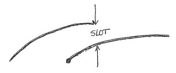
This is how the jib is used to generate more power for the mainsail: by using it to accelerate the airflow on the leeward side of the mainsail. The space, and overlap, between the leach of the jib and the luff of the main is called "the slot". Managing the slot is accomplished principally through the placement of the jib fairleads and jib sheet tension.
