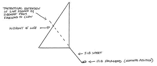
From that point, it is a matter of seeing what works best. Generally, the fairleads will be move aft of the neutral position when going upwind and forward of the neutral position when going offwind. Adjustment when sailing close hauled should be focussed on reducing backwinding of the main when both sails are properly trimmed for heel. That said, some backwinding of the main should remain about 36" above the boom and about a foot aft of the mast.
