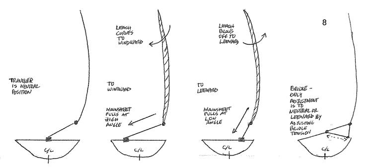
The other effect the mainsheet can have on mainsail shape is to flatten the lower mid portion of the sail. As the mainsheet is pulled in, it starts to exert a downward force on the middle section of the boom. If the boom is not stiff enough to resist this force, it will bend. As the boom bends, it will stretch the sail downward, reducing draft. This is not desirable and is one of the reason modern booms are quite stiff.
