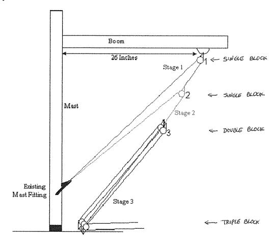
Combined with modern extremely stiff booms, the increase in purchase brought a fundamental change in role for the boom vang. Today, on high performance dinghies, the boom vang is as key as the mainsheet to controlling the shape, and thus the power, of the mainsail.
