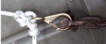
Figure 3 Spring Line anchor point in boat
