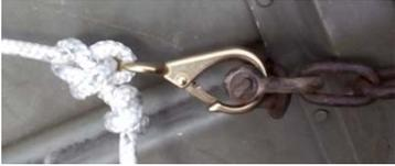
12. Connect the bow and stern whip lines to their respective anchor points in the boat. Ensure that the whip line *slide-lock* bar is approx. 1 foot up the whip line rope.
